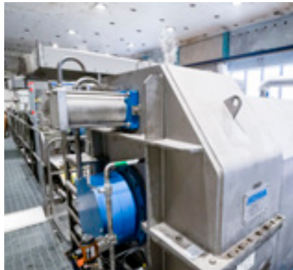
As well as the two twin wire presses, Holmen Paper Hallsta also utilized a second-hand ANDRITZ pulp screw press to improve pulp washing for PM12.
